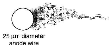
Figure 8.3. An orthogonal view of an avalanche triggered by a single electron. The density of the shading indicates the concentration of electrons formed in the avalanche. After Knoll [2000].
