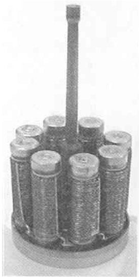
Figure 12.13. The BASE cells and sodium artery in an AMTEC converter. Each cylindrical cell is 1 cm in diameter with a 2.5 cm active electrode length. Courtesy of Advanced Modular Power Systems, Inc.
